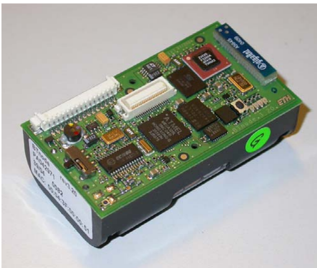
Figure 2.11 The BT Node (BTnode 2008).
