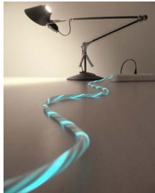
Figure 18. An illuminated electrical cord by The Interactive Institute, Sweden makes the users aware of their consumption. (Mynewsdesk 2006)
