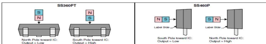
Figure 11. Poles of the magnetic sensor (Honeywell SS360PT/SS460P 2013).
