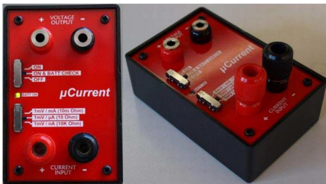
Figure 8. The \mu Current active current sensor for multimeters and oscilloscopes
