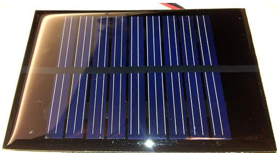
Figure 12. The 92x61x8 mm, 0.45 W solar cell
