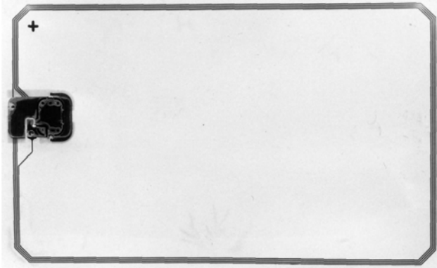
Figure 21. An inlay foil for a contactless smart card with inductive coupling using an etched coil
