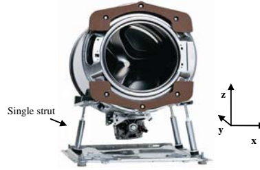
Fig. 2 The three-strut concept
