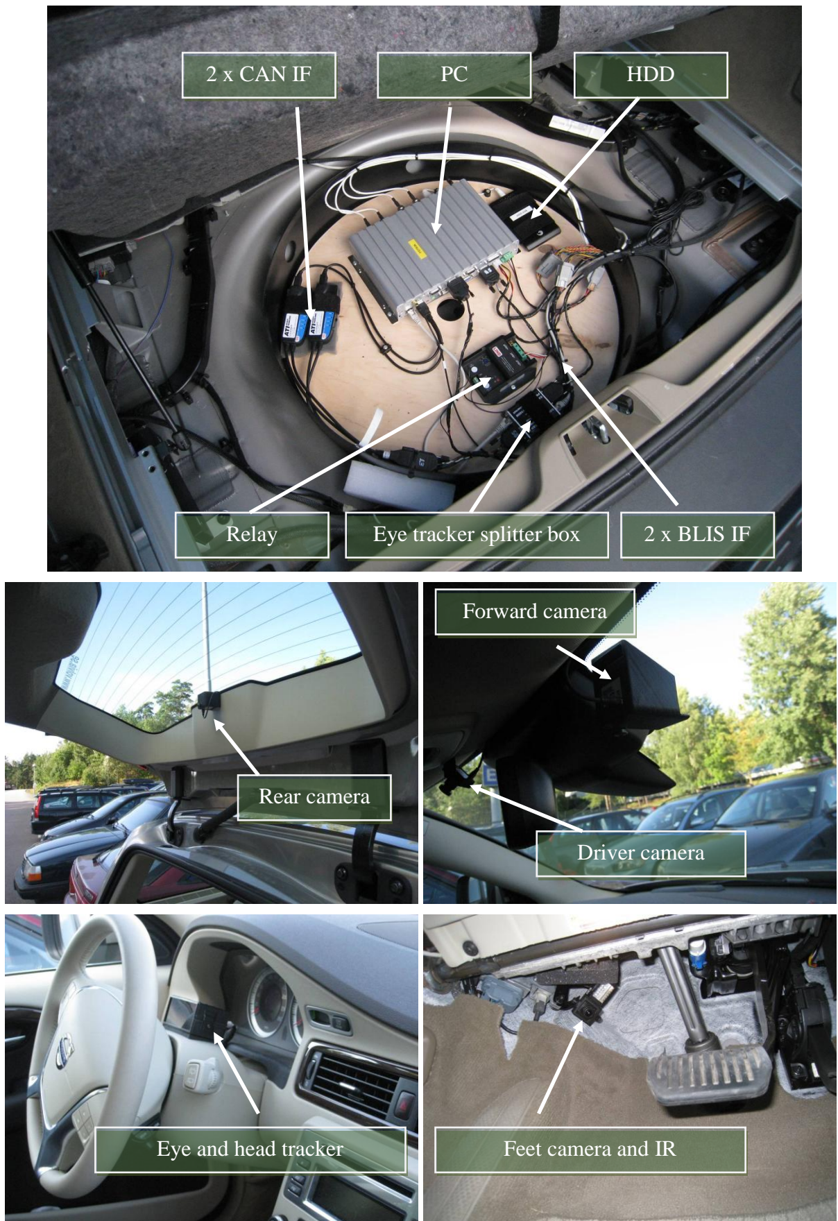
Figure 17: Swedish VMC - Placement of DAS including extra sensor and cameras.
