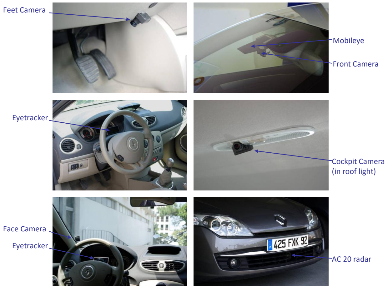
Figure 16: French VMC - Placement of extra sensors and cameras.
