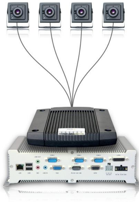
Figure 14: Video logging system at French VMC.
