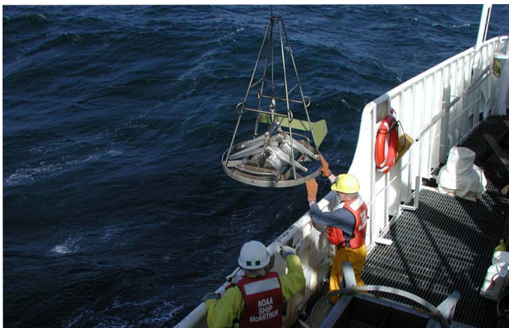
Deploying a dual Van Veen grab sampler from the RV McArthur II.
