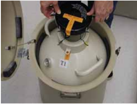
Figure 4.8 Dry shipper. Note lid and canister alignment are critical to ensuring proper seal.
