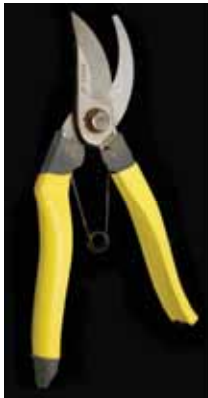
Figure 4.6.6.1 Clippers used for sampling branching corals
