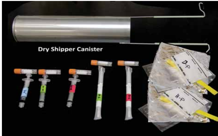
Figure 4.7.2.3 Summary of samples to be frozen showing the packaging used for freezing.
