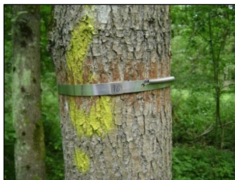
Figure 2.6: Tree with installed dendrometer band
