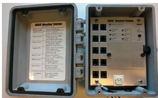
b) HOBO® Weather Station H21-001
