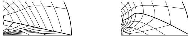
Fig. 13. An inner boundary of a multi-patch configuration. To the left the initial parametrization, to the right the parametrization obtained by minimizing the Winslow functional.
