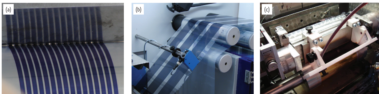
Fig. 6 (a) Photograph of the standing meniscus during slot-die coating of the active layer of the OPV comprising many very tightly spaced stripes. (b) A total of 48 stripes (3 mm wide spaced by 1 mm) are coated simultaneously. (c) Knife coating with the open ink reservoir and the manual feed hose.
