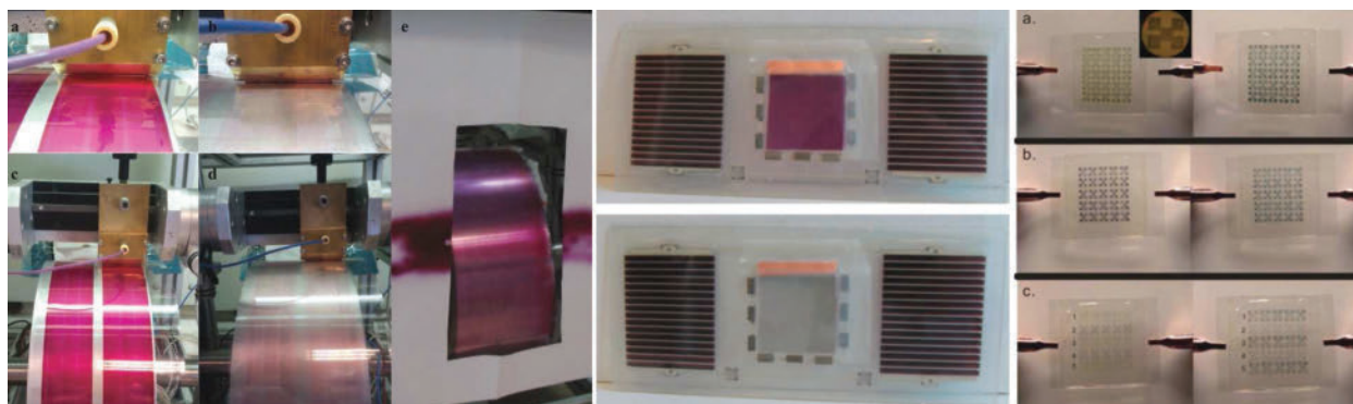
FIGURE 10 Left: Picture of slot-die coating and spray coating of polymer electrochromes on a single roll system. Middle: Pictures of an integrated polymer electrochromic/polymer solar cell demonstrator. Right: Examples of inkjet printed electrochromic devices. Reprinted from Ref. 74 and Ref. 81, with permission from 2012 Wiley Periodicals, Inc and The Royal Society of Chemistry 2008, respectively.
