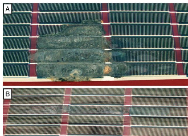
Figure 2. A) Photograph of large-scale defects induced by delamination from the bottom side. Water ingress leads to a propagating area of inactive solar cells. B) A long scratch caused during the installation affects three solar cells. Water and oxygen ingress changes the visual appearance of the cells.
