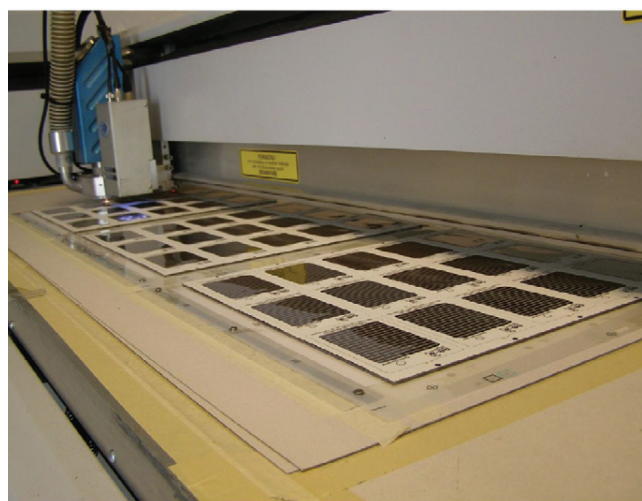
Fig. 15 Illustration of the OE-A demonstrator for 2011 and an example of the laser cutting the processed sheets into the final product.
