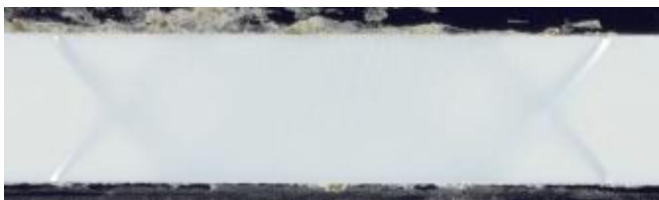
Fig. 6. Cross-polarised transmission optical image of the gauge region of the plane-strain compression test of the epoxy polymer modified with 10 wt% S-CSR particles loaded to just after the yield point.
