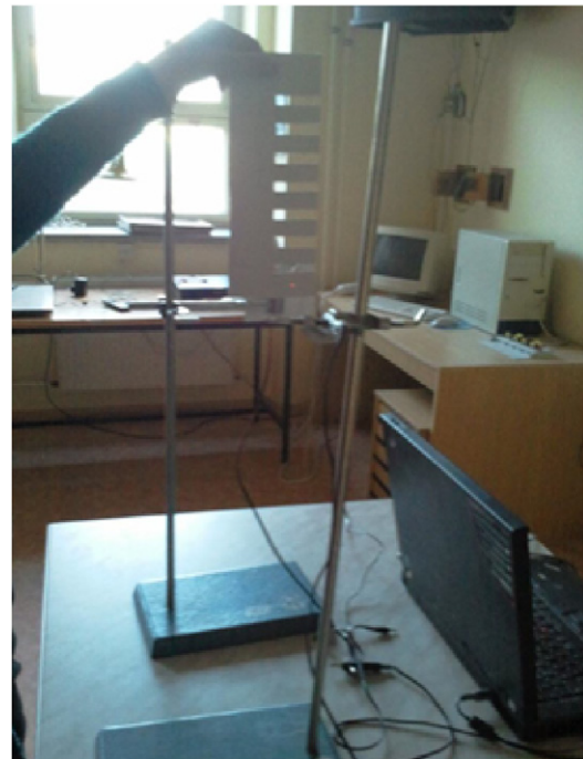
Figure 2. Free fall of a cardboard comb.
