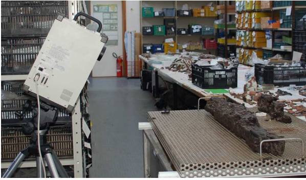
Fig. 3. Minolta ® Vivid 900 from the 3D Laboratory of SIBA of the University of Salento that was used for the 3D laser scans.
