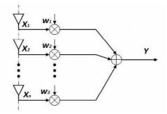
Figure 3. Narrowband Beamformer.
