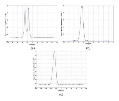
**Figure 4.** (a)  $DOA_1 = -30^\circ$ ,  $DOA_2 = -15^\circ$ ; SNR = 15 dB. (b)  $DOA_1 = -30^\circ$ ,  $DOA_2 = -25^\circ$ ; SNR = 15 dB. (c)  $DOA_1 = -30^\circ$ ,  $DOA_2 = -25^\circ$ ; SNR = 5 dB.
