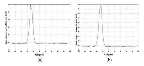
**Figure 6.** (a)  $DOA_1 = -30^\circ$ ,  $DOA_2 = -25^\circ$ ; SNR = 5 dB; samples = 100. (b)  $DOA_1 = -30^\circ$ ,  $DOA_2 = -25^\circ$ ; SNR = -5 dB; samples = 1024.
