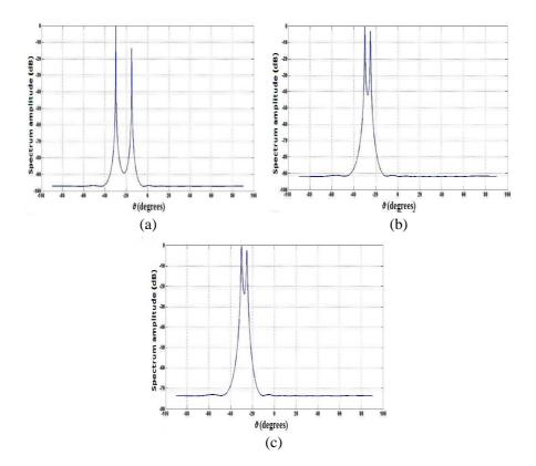
Figure 5. (a)  $DOA_1 = -30^\circ$ ,  $DOA_2 = -15^\circ$ ; SNR = 15 dB. (b)  $DOA_1 = -30^\circ$ ,  $DOA_2 = -25^\circ$ ; SNR = 15 dB. (c)  $DOA_1 = -30^\circ$ ,  $DOA_2 = -25^\circ$ ; SNR = 5 dB.
