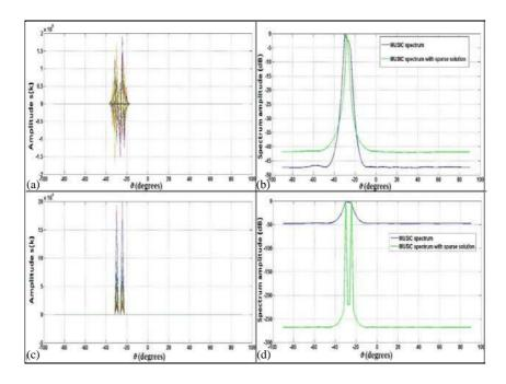
**Figure 10.** (a) Iteration #2: Tikhonov solution. (b) MUSIC spectrum without sparse solution vs. MUSIC spectrum with sparse solution. (c) Iteration #5: Tikhonov solution. (d) MUSIC spectrum without sparse solution vs. MUSIC spectrum with sparse solution.
