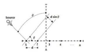
Figure 2. Linear array of *n* antenna sensors.
