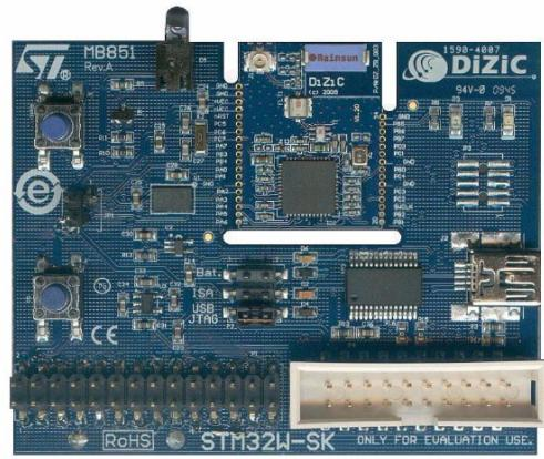
Fig. 1. The MB851 evaluation board.
