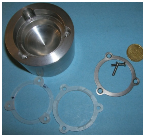
Figure 3: Mounting System Screws and rings.
