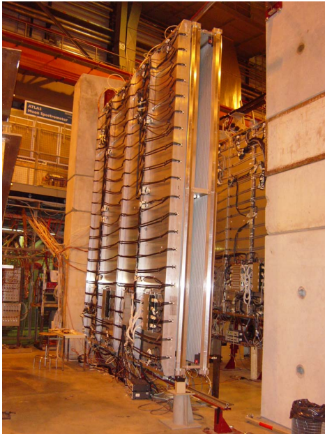
Fig. 3. Particular of the set-up of the Muon Barrel trigger at the H8 test beam. In the foreground the BOL chamber with high- p_t trigger electronics mounted on, the BML station is visible in the background.
