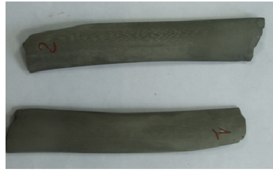
Fig.5. Chemically etched, defect free SX blades cast from TiO 2 doped silica cores
