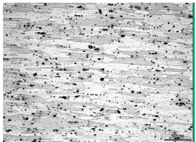
Fig. 4 – Initial microstructure of the studied alloy revealing the classical elongated grains belonging to the rolling operations.
