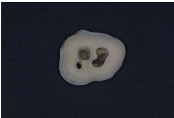
Figure 4-2 Dentine disc prepared by segmentation of teeth samples using a diamond wheel saw, prior to dentine hardness measurement and histological studies of dentine.
