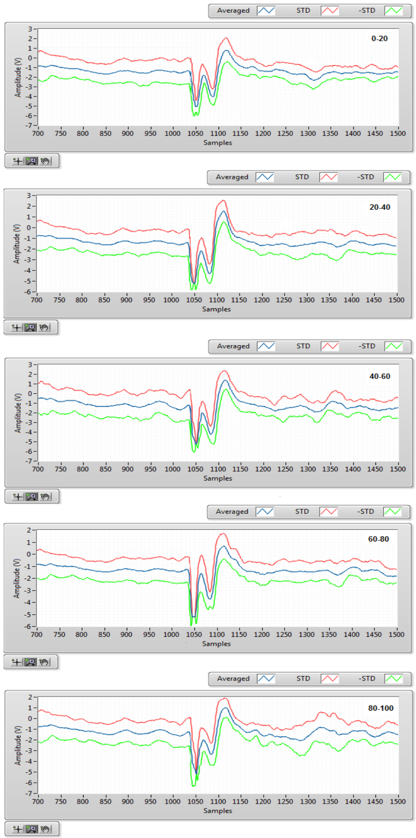
Figure 5. 15: Mean EMG signal before and after the stimulation averaged by a moving window of 20 revolutions, revolution numbers are at the top right corner of each graph.
