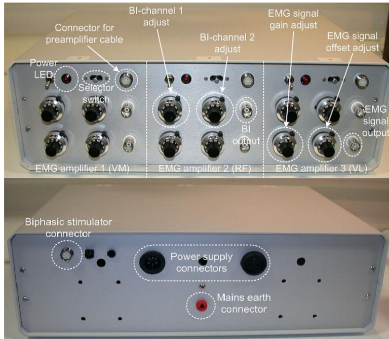
Figure 4. 34: The front and back panel of the EMG amplifier with current conveyer.
