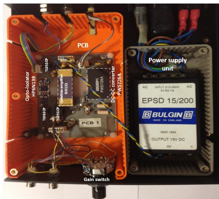
Figure 4. 17: The inside of the isolation amplifier, left half is a PCB containing all the ICs and the right side is the battery. Both the PCB and the power supply unit are fixed in plastic boxes.
