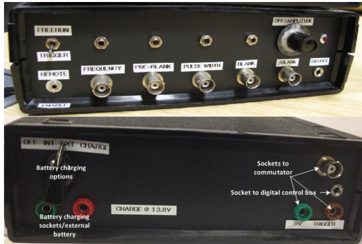
Figure 4.20: The stimulator front and back panels.
