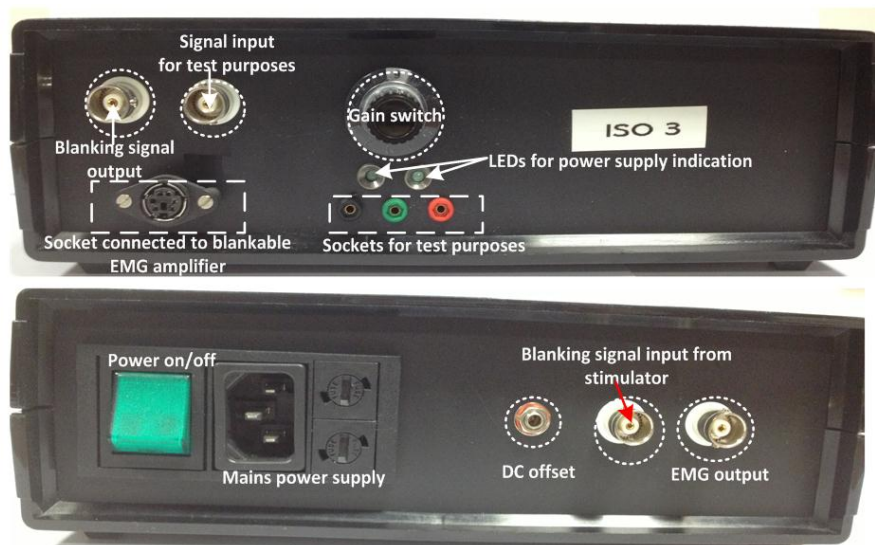
Figure 4. 16: The isolation amplifier box front panel (above) and back panel (below).
