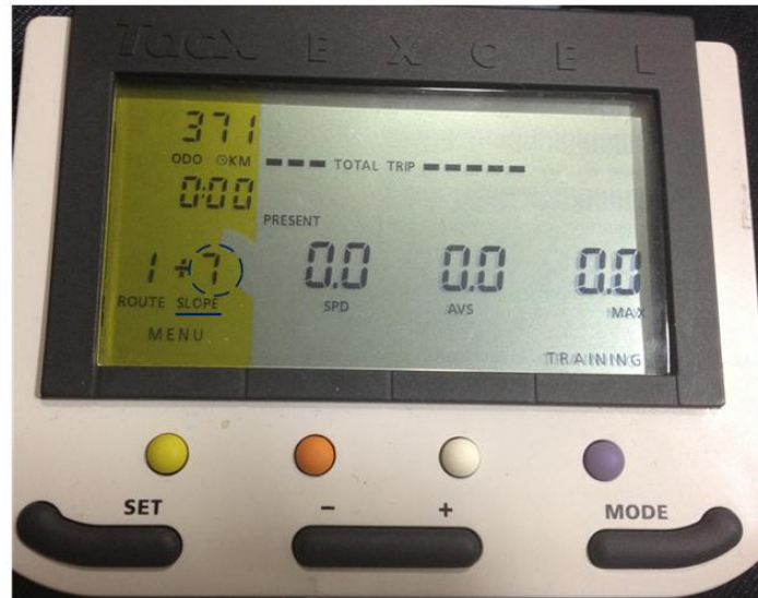
Figure 4. 3: The cycling computer to control the resistance applied to the back tyre of the trike, the slope (effort level) was circled.
