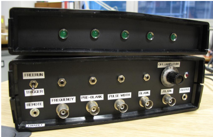
Figure 7. 3: A photo of the 5 channel control box sitting on top of the stimulator.
