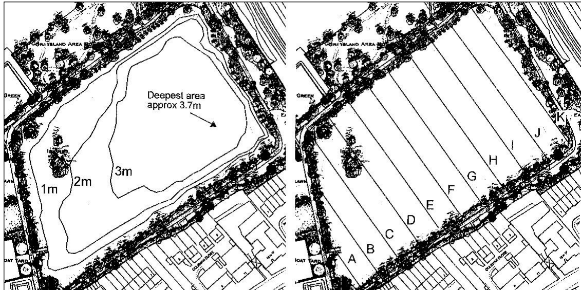
Figure 2.2 – Left - depth contour map of South Norwood Lake; Right - the location of transects used for the assessment of water and sediment depths in 2000 (from EAC Ltd, 2000).
