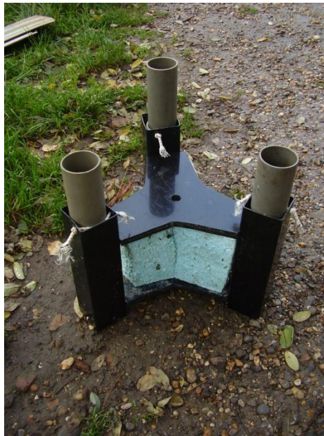
Figure 5.2 – one of the two sediment traps installed at the Vale of Health Pond
