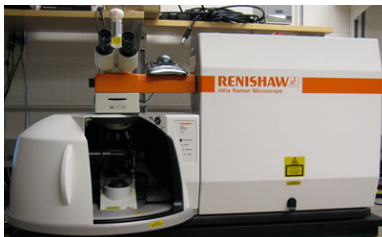
Figure 3.5: The Renishaw inVia Raman microspectroscopy apparatus.
