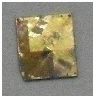
Figure 4.6: Photograph of the circuit-side of a decapsulated SIM chip still retaining a large amount of EMC on surface of topside circuit.
