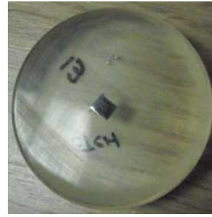
(b) Resin test with 5:2 mix ratio
