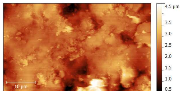
Figure 7.8: Topography map obtained from a grain in sample set 3 showing upturned plates formed by wind abrasion. Scan size 30\mu\text{m} \times 50\mu\text{m} .
