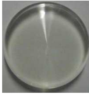
Figure 4.11: Photograph of a superior resin cast created through mixing with a magnetic stirrer and agitating for short bursts in an ultrasonic bath.
