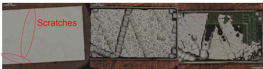
Figure 4.20: The effect of surface scratches on the choline hydroxide etching. 2.5× optical zoom. From left-right: 0 mins, 40 mins, 65 mins. From [8].
