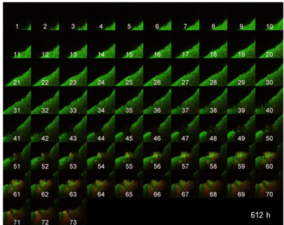
Figure 4.23. Individual optical sections of biofilms sampled at 612 h from both experiments 4 and 5. Numbering is from 1 at the apex in 1 \mu\text{m} increments until the titanium surface is reached.
