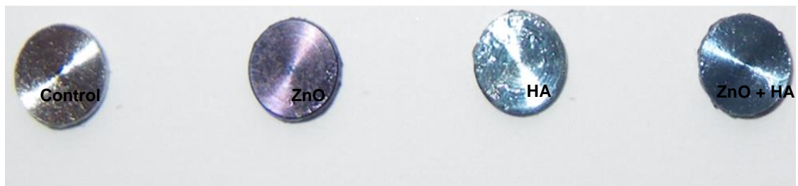
Figure 8.7. The surface colour of the Ti coated discs after 600°C treatment. ZnO coating become purple, HA become dark blue and combined ZnO + HA become blue/grey colour).
