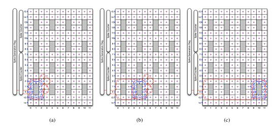
Figure 5.10: Three examples of test cases for testing dendrite signal routing around soma cells on the cortex. The particular shape of the dendrite in (a) and (b) tests all possible different switch states through a single dendrite loop.
