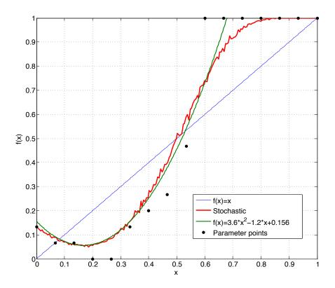
Figure 4.4: Simulation results of a 16x4-bit stochastic function generator with parameters tuned to approximate the function  $f(x) = 3.6x^2 - 1.2x + 0.156$  (shown in green). The red curve shows the probability of the function generator output bitstream against the input value (x). Intersection points of the blue line (f(x) = x) and the update function determine the resting (x = 0.1) and threshold (x = 0.5) potentials respectively.
