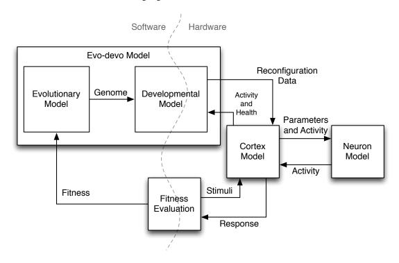
Figure 7.1: An abstract data flow diagram showing the interactions between different models in the system and demonstrating the hardware-software partitioning problem.
