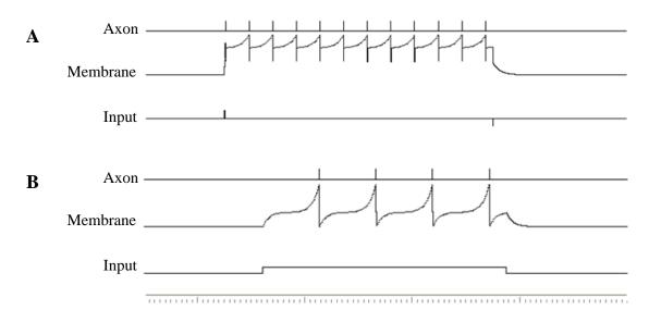
Figure 4.9: Traces of the input current, membrane potential, and the axon output of the digital neuron in the first experiment: A) Bistable behaviour ( $u_{reset} = 17000$ ). B) Monostable behaviour ( $u_{reset} = -16384$ ).
