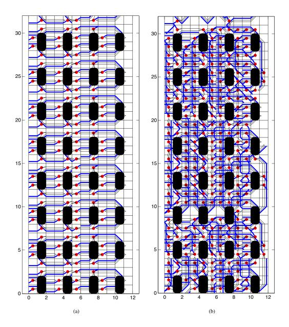
Figure 6.22: Two example best fit microcircuit phenotypes after the fitness convergence of the example run (at about 4000 evaluations). (a) The fittest microcircuit of the population at generation 131 with eight clusters of four neurons. (b) The fittest microcircuit of the population at generation 141 with larger and more complex clusters but with the same fitness (mean clustering coefficient to characteristic path length) ratio as (a) equal to 1.17.
