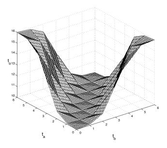
Figure 7.4: A 3D plot of the desired output timing  $(t_o)$  as an interpolated XOR function of two input spike timings  $(t_a \text{ and } t_b)$ .
