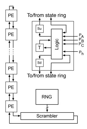
Figure 4.2: Left: general design of a distributed stochastic model consisting of a random number generator (RNG), a scrambler, and a number of processing elements (PE). Right: internal structure of a processing element (PE). Su, Sd, and T are the State up, State down, and token flip flops respectively.
