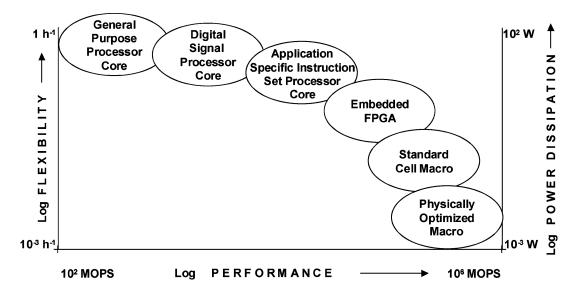
Figure 2.3: From[38], flexibility, power dissipation and performance of different digital design approaches. Flexibility is measured in the reciprocal of the design time.
