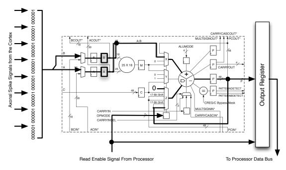
Figure D.1: Block diagram of the Spike Counter module with configuration of the DSP block as eight 6-bit counters.
