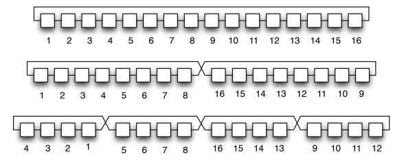
Figure 5.16: Solution to wrap-around wire delays in a 16 node ring network. The top connectivity pattern involves a very long wire between the first and last nodes while other links are very short. In the second pattern this delay is divided in half between two wires by flipping right half of the nodes. In the third pattern a quarter of the nodes at each end of the ring are also flipped again to cut the delays in half again.
