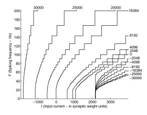
Figure 4.10: F-I curve of the digital neuron using different values of  $u_{reset}$  showing class 1 and 2 excitability.
