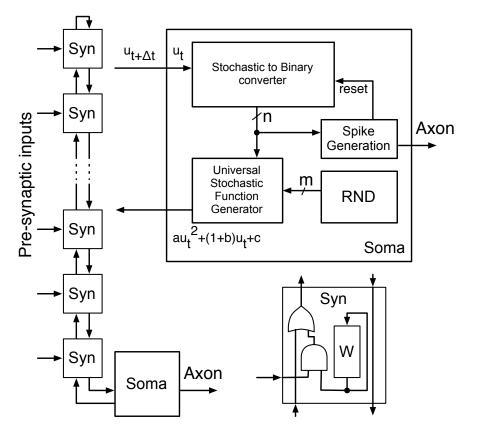
Figure 4.3: Left: General design of a centralised stochastic model. Right: Internal structure of the soma and synapse units. RND represents a source of random bitstreams with specific probabilities.
