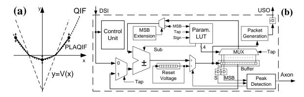
Figure 4.6: (a) The PLAQIF model approximates the QIF model (the dotted curve) with a piecewise linear function by modulating the V-shape function V(x). The control points (arrows) can be moved by tuning the parameters. (b) Soma unit
