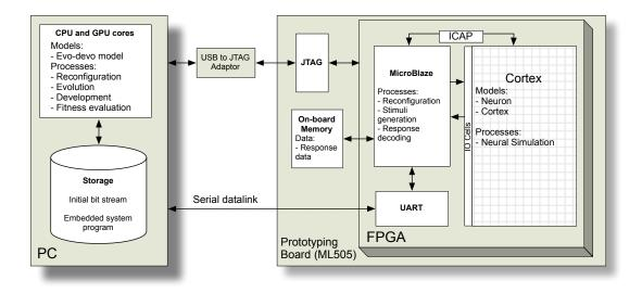
Figure 7.5: A block diagram of the integrated system of the case study showing the connectivity of the main components (PC and FPGA) and mapping of the modules and processes to these components.
