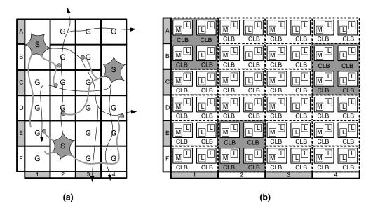
Figure 5.6: (a) Symbolic view of the example microcircuit in a 4x6 cortex. (b) Assignment of FPGA CLBs to glial and soma cells.
