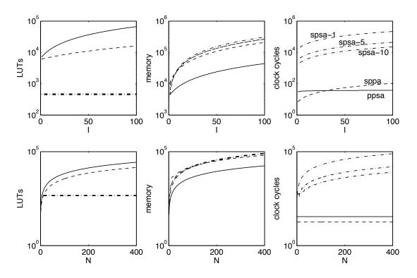
Figure 2.8: From [330], comparison of hardware resources and speed of different architectures (the SPSA architecture with 1, 5 and 10 PEs) with different number of inputs (I) and number of neurons (N).
