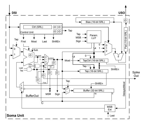
Figure 5.14: A detailed diagram of the revised soma unit showing the bias register, serial adder and padding shift register that were added to the soma unit. The global reset and clock signals are not shown here.
