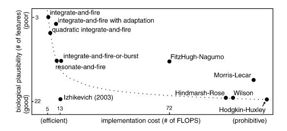
Figure 2.5: [169] Number of biological features of the spiking neuron models against number of floating point operations needed for simulation of one millisecond of neuron activity with each model [169] based on Table 2.1.
