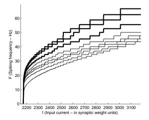
Figure 4.11: The effect of moving the middle control point (of figure 4.6(a)) on the F-I curve of the digital neuron. The bold lines are results of the middle point higher than zero.
