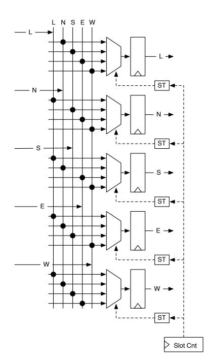
Figure 5.2: The circuit to be added to each PE for time-multiplexed switching of a 2D mesh network (From [328]). L, N, S, E, W respectively present links to and from Local PE, North, South, East, and West nodes. ST represent a Scheduling Table.
