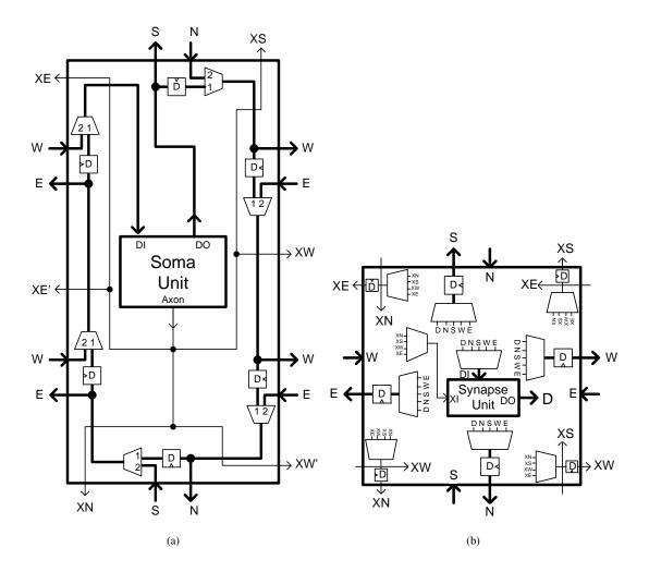
Figure 5.5: (a) Internal Architecture of soma cell. (b) Internal architecture of glial cell
