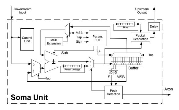
Figure 5.12: Block diagram of the revised soma unit showing the bias register, and the delay block that were added to the soma unit. The global reset and clock signals are not shown here.
