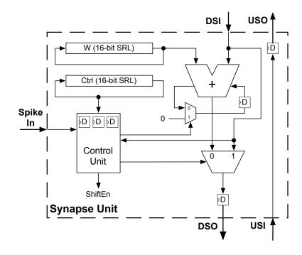
Figure 4.8: Detailed block diagram of the synapse unit design.
