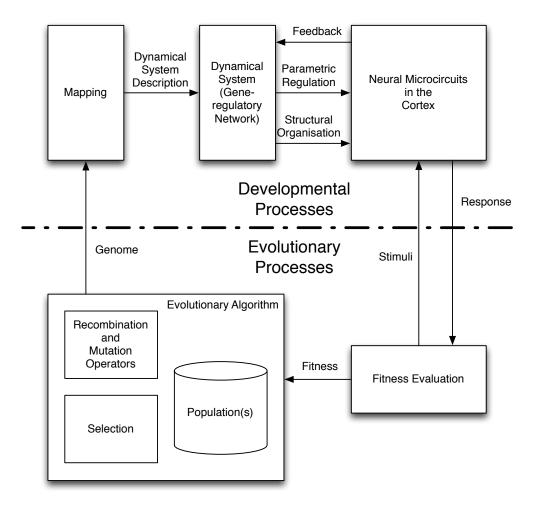
Figure 6.1: Different functions of the evo-devo model and their interactions. Evolutionary and developmental processes are separated from each other. Both processes need to share the same genetic representation.
