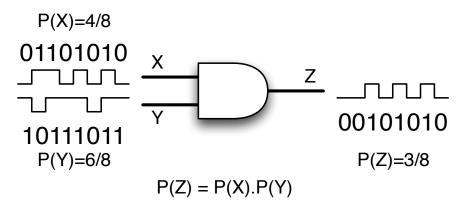
Figure 2.7: A simple example of computing product of two stochastic signals represented by 8-bit long random bitstreams using a single AND gate.
