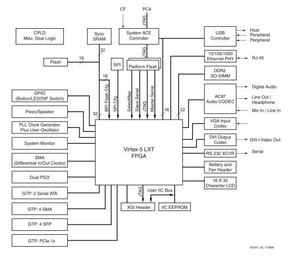
Figure 3.4: The ML505 platform block diagram.
