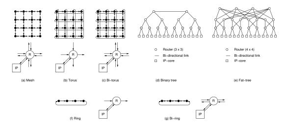
Figure 5.1: Common NOC topologies along with their router(R) and PE (IP) connections and ports (From [328]).
