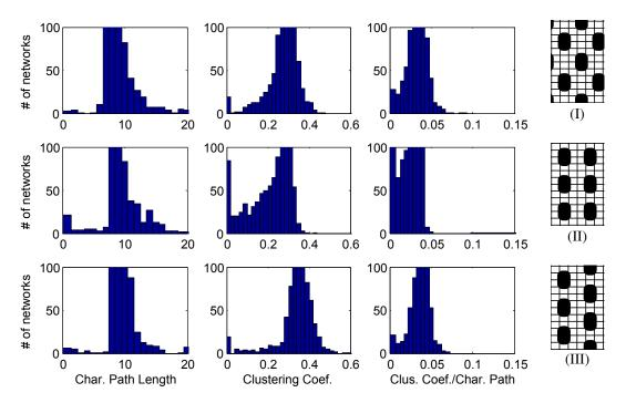
Figure 6.13: Distribution of the characteristic path length, clustering coefficient, and their ratio for 1000 developed networks using randomly generated genomes with 3 different neuron placement patterns (I, II, and III).
