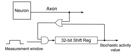
Figure 5.3: An example of a circuit that can be used to gather stochastic measurements of the activity of a neuron over a measurement period.
