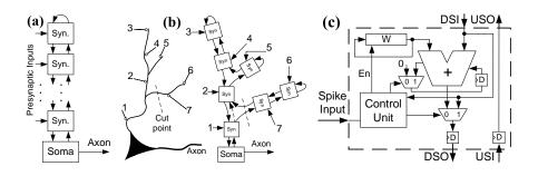
Figure 4.5: a) General architecture of the digital neuron (Syn=synapse) b) Example of the dendrite structure and its adaptability (c) Synapse unit architecture.
