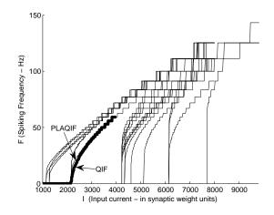
Figure 4.12: F-I curve of the digital neuron using different parameter settings for  $p_{i,j}$  and  $s_{i,j}$  keeping  $u_{reset} = -16384$ along with the F-I curve of the QIF model of equation 4.16 superimposed in bold.
