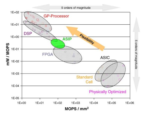
Figure 2.2: From [278], energy and area efficiency of different digital design approaches.
