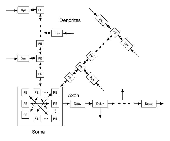
Figure 4.1: Abstracted general architecture of a neuron as an aggregation of processing elements (PE), synapses (Syn), and delay elements (Delay).
