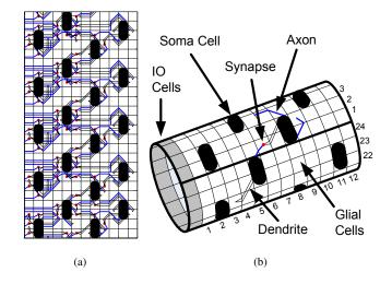
Figure 5.4: (a) A sample 12x24 cortex with 20 neurons. (b) The 2D cylindrical structure of the cortex.
