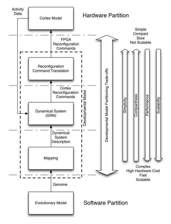
Figure 7.3: Developmental model partitioning trade-offs depicting the growth of different factors based on the partitioning boundary between hardware and software components of the system. The stroke dash lines represent some of the different options for the partitioning of the developmental model between hardware and software components.
