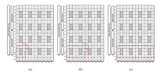
Figure 5.9: Three examples of test cases for testing axonal signal routing around soma cells on the cortex. The particular shape in (a) and (b) insures that every different switch state is at least once tested through an axonal path.
