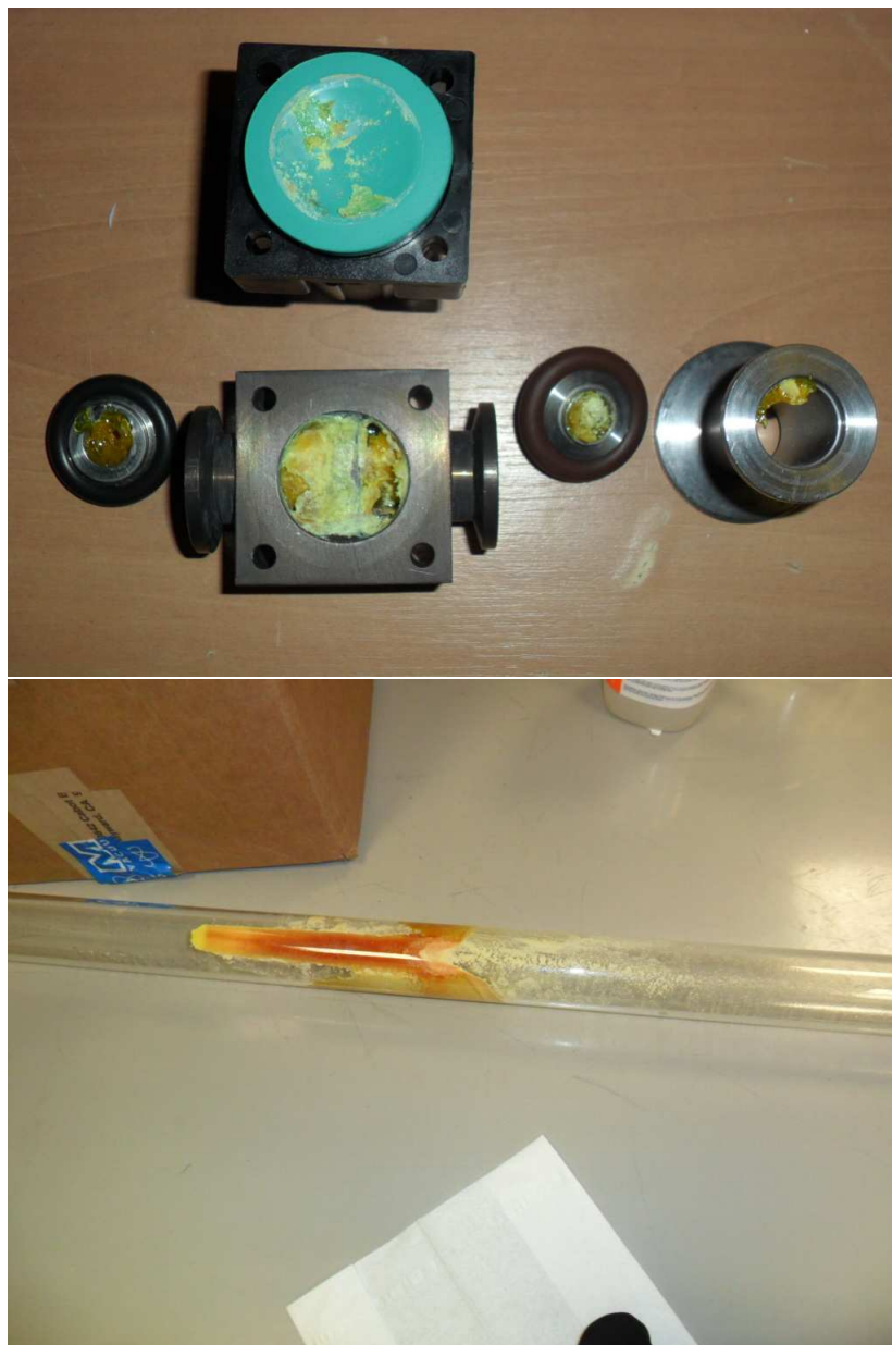
Figure 6.2: Sulphur deposition in the valves and on the inner side of the pyrex cell.
