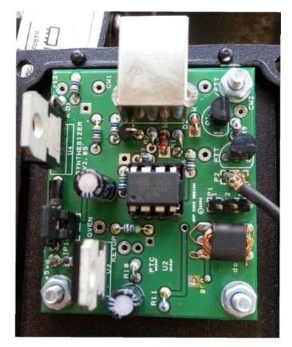
Figure 4.4: USB controlled oscillator
