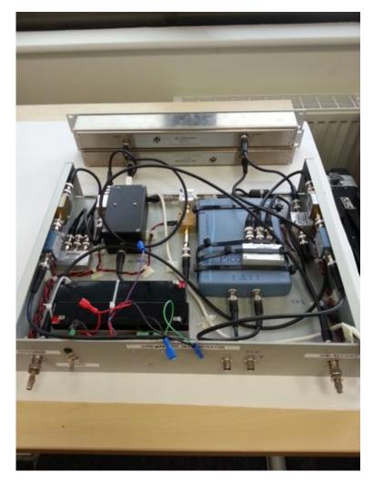
Figure 4.14: Completed receiver - under the lid
