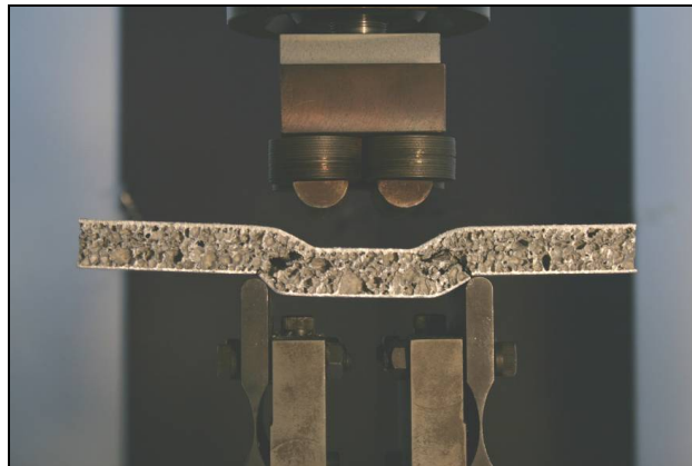
Figure 2: Failure mode for AFS-1 specimen.
