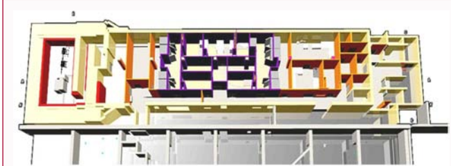
Figure 4: The layout of the Radiopharmaceuticals Production and Research Centre. The radioisotopes produced by the proton or deuteron beam from the PETtrace cyclotron (left of the figure) are transferred to one of the chemistry laboratories: L1 serving for the routine production of Fluoro-Deoxy-Glucose (FDG) or L2 devoted to research activity with ^{11}\text{C} , ^{15}\text{O} or ^{18}\text{F} radioisotopes. The quality control area (right of the figure) is also divided into two parts: for testing regularly produced FDG and for radiopharmaceuticals in the research stage.
