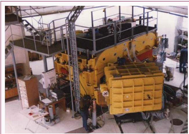
Figure 2: The K=160 heavy ion cyclotron, accelerating gaseous and metallic ions with masses up to 40 and energies up to about 10 MeV/nucleon.
