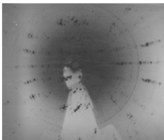
Figure 4.2 The Laue diffraction pattern of single crystal Nb 2 O 5 collected on crystal as-grown.
