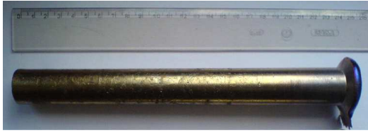
Fig. 1. A view of ingot of studied NiTi alloy.
