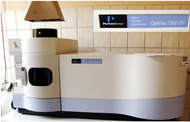
Fig. 2. Inductively coupled plasma optical emission spectrometer ICP-OES Optima 7300 Dual View Perkin Elmer.
