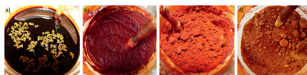
Figure 3. The co-precipitation method of the PFN material (PFN-c); a) the solution with precipitation process, b-c) the solvent vaporization supported by IR rays, d) PFN-c powder.
