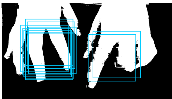
Figure 7. Image I^S , where squares indicate the location of the right hand, determined with the use of n = 10 patterns.
