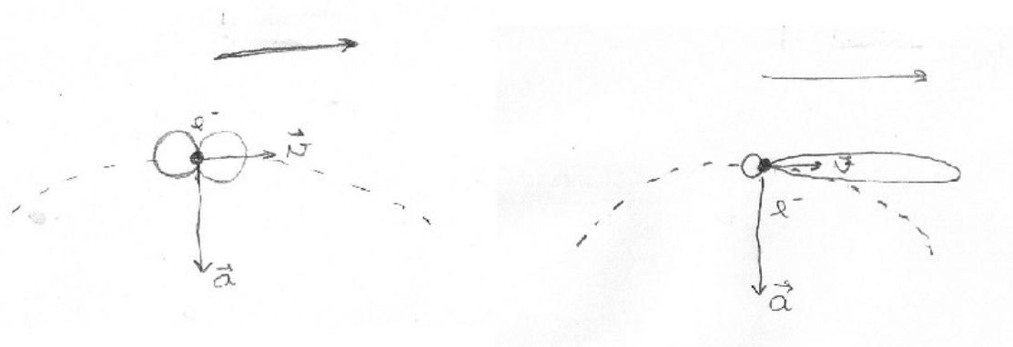
Fig. 9: The effects of beaming on the Synchrotron radiation. On the left the schematic of the radiation of a Cyclotron (the classical equivalent to Synchrotron). On the right the Synchrotron radiation subjected to beaming. The arrows above the schematics indicate the direction to the observer.
