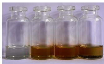
Figure 4. Samples of sulfolane, from the left: pure sulfolane, sulfolane after the experiment at 95 °C (details in the experimental section) with the addition of 2%, 4% and 6% vol. water, respectively.
