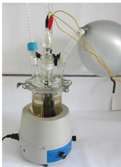
Figure 6. The complete laboratory setup for sulfolane corrosivity tests.
