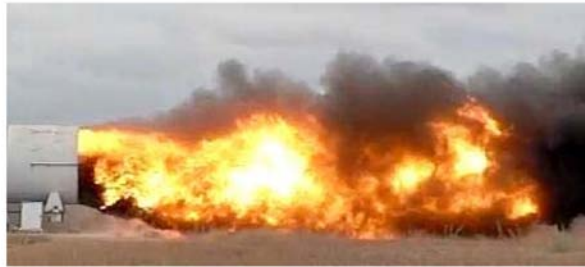
Figure 4: Demonstration of a propagating coal dust explosion at the Kloppersbos facility (reproduced with permission from Humphreys et al. (2010)).
