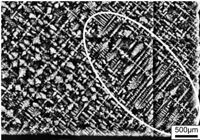
Fig. 8. SEM micrograph (BSE technique) of the blade root dendritic structure in area 4 (Fig. 3)
