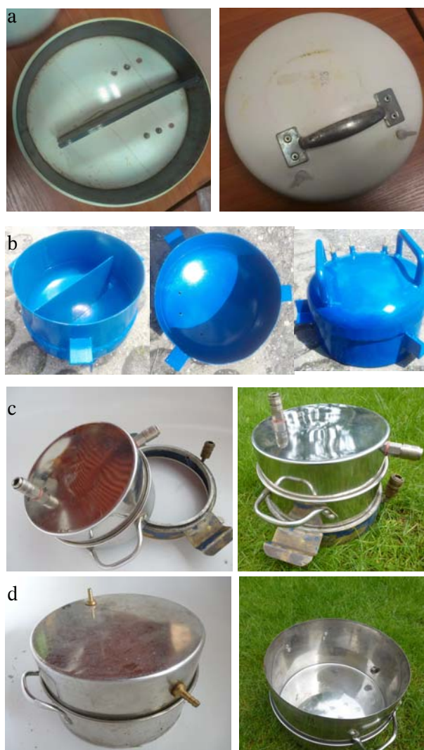
Fig. 2. Different accumulation chambers used in the present studies: (a) from the University of Silesia (Durrigde, USA chamber) with the partition with V/S = 0.110 \text{ m} ; (b) from the University of Silesia with and without the partition with V/S = 0.129 \text{ m} ; (c) from the Institute of Nuclear Physics PAN without the partition with V/S = 0.120 \text{ m} , and (d) from the Institute of Nuclear Physics PAN without the partition with V/S = 0.15 \text{ m} .
