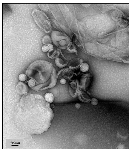
Figure 2. Transmission electron micrographs of liposomes containing cytarabine and methotrexate ( L_{DPPC/AraC/MTX} ) obtained by the modified reverse-phase evaporation method (mREV), negatively stained (2% uranyl acetate solution) on a carbon-coated copper grid, magnification: 50,000 times; at room temperature.
