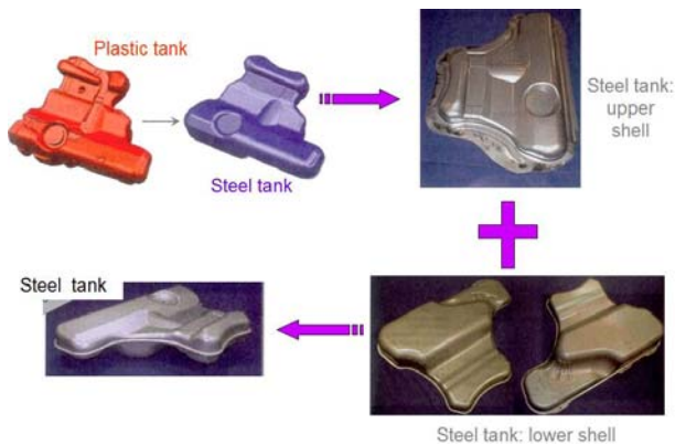
Figure 8: from the plastic tank to the parted steel tank.
