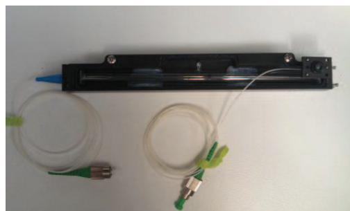
Figure 9 - A pre-filled methane gas cell from Wavelength References Inc. (Shemshad, 2012)
