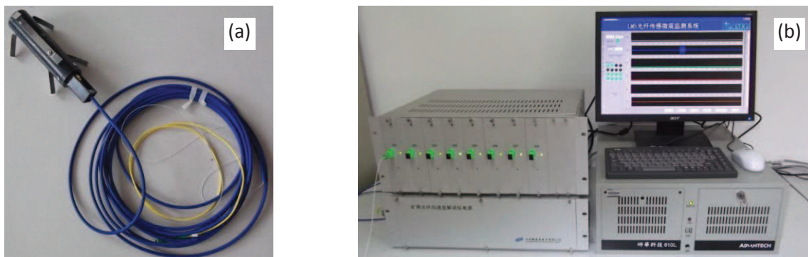
Figure 19 - (a) Micro-seismic acceleration sensor (b) Micro-seismic demodulator and data processor
