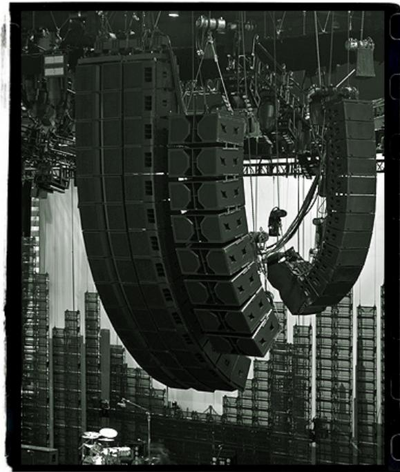
Figure 3.2: Example of a loudspeaker array
