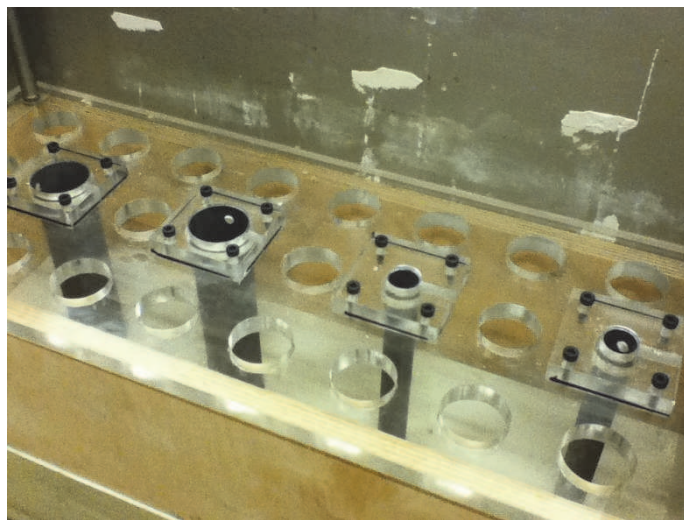
Figure 6. Perspex template used to hold casing vertical.
