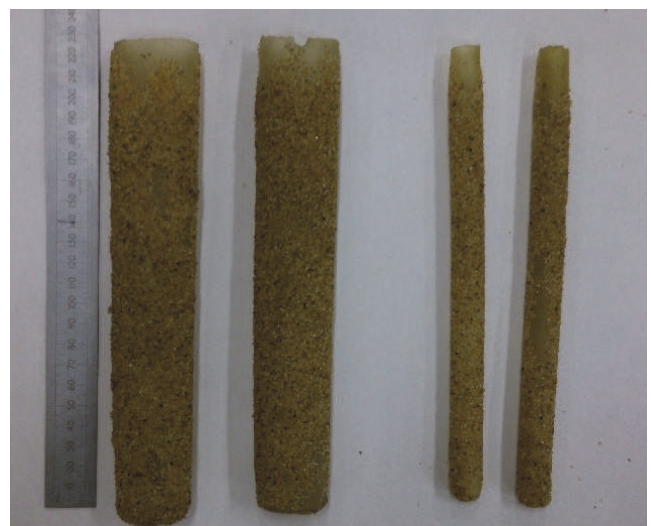
Figure 3. Sand covered latex membranes.
