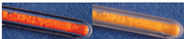
Fig. 10 Digital pictures of crystals of 5 at room temperature (left) and after immersion in liquid nitrogen (right).
