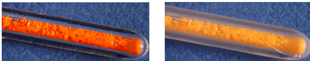
Figure 3.13. Digital pictures of crystals of 25 at room temperature (left) and after immersion in liquid nitrogen (right). [Pub 2]
