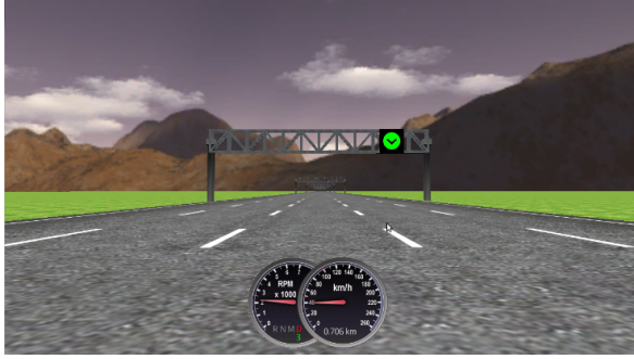
Figure 2: Driver’s view during experiment. The green signal on the signal-bridge indicates the target lane.
